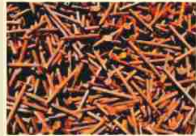
Fig (3-10) Rusty nails after exposure to moisture
